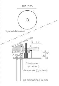
Measure and mark the light fixture canopy position on the ceiling.
