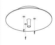
Anchor canopy into the plywood backing using the fasteners provided.
