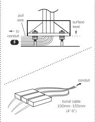
After each branch is installed, feed pull wire through pre-laid conduit to the driver (power supply) location.
