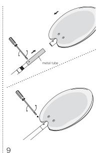
Remove the metal tube at the end of each branch by unscrewing the set screw.
