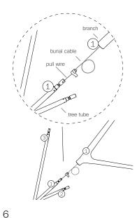
Matching the branch number with the tree tube number, secure the burial cable of each branch to the end of the pull wire with tape or
