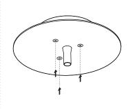
Anchor canopy into the plywood backing using the fasteners provided.
