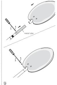
Remove the metal tube at the end of each branch by unscrewing the set screw.
