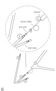
Matching the branch number with the tree tube number, secure the burial cable of each branch to the end of the pull wire with tape or other temporary means.
