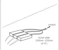
After each branch is installed, feed pull wire through pre-laid conduit to the driver (power supply) location.
