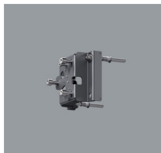
34953.000 Attachment for upright supporting pole \varnothing 60–89mm. Housing: stainless steel. Graphit m, powder-coated. Clamping plate or second attachment for fixing to be ordered separately. Upright supporting pole \varnothing 60–89mm to be ordered separately. Weight 1.00kg
