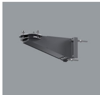
34955.000 Cantilever arm for standing luminaire installation on upright supporting pole \varnothing 60–89mm or wall. Housing: stainless steel. Graphit m, powder-coated. Clamping plate or second cantilever arm for fixing on upright supporting pole to be ordered separately. Upright supporting pole \varnothing 60–89mm to be ordered separately. Weight 2.20kg
