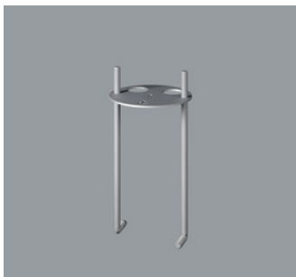
33979.000 Concrete anchor Mounting plate with threaded bar and fixing nuts M6. Individual parts to be assembled on-site. Weight 0.25kg
