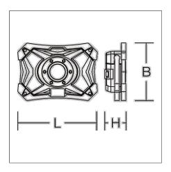
Mobile, mains-independent battery-operated work light. Housing made of robust die-cast aluminium with soft edge protection made of TPE (thermoplastic elastomer). Highly efficient COB LED. Beam angle adjustable with handle. Multi-level switchable with push-button. (OFF, 25, 50, 100%). Built-in Li-Ion battery. (4.400 mAh). Operating time up to 10 hours. Charge status display. With powerbank function for charging external equipment. Incl. charging cable. (USB-A > Micro-USB)
