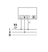
$Standard\ operation\ with\ optional\ parallel\ connection\ of\ automatic\ luminaires.$
