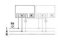
Standard operation with optional parallel connection of automatic luminaires.
