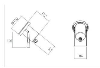
IT: Adjustable outdoor light fitting with a typical linear and functional design, entirely made of stainless steel. The faceted specular reflector for different light beams makes it versatile to use, both for spot lighting of monuments and facades and for gardens and outdoor architecture.Body and closure ring in AISI 304 stainless steel, ransparent tempered glass, silicone rubber gasket.Facetted specular reflector for 36 ° / 24 ° / 12 ° light beam.Supplied complete with integrated driver.
