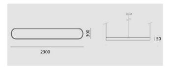
IT: Minu-R is a collection of decorative lighting rings with direct or internal light. It can offer such elegant and light design, with great scenic impact; it is the ideal choice for offices, residential and commercial environments. Structure in powder coated curved extrusion of aluminium alloy with opal diffuser. 4000K or 3000K white tone. Powers from 50W/1150mm up to 95W/2300mm. Suspension kit to be ordered separately. On-Off or Dali Driver included in the ceiling cup.
