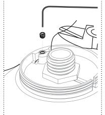
Once the pendant is positioned at the desired height, tighten the set screw to lock in the aircraft cable.
