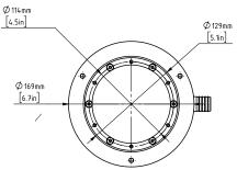
Installation housing AXMLN\*fits 1m (3,3') cable Liner pool installation
