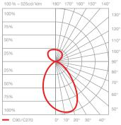
wide light beam (up and down), beam angle approx. 80° directed (down)
