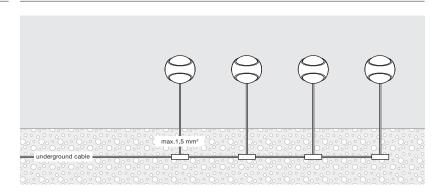
through-wired with plug in terminals
