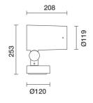
Spotlight with base - Warm White Led - integrated electronic control gear - Super Spot optic Photometric data for this product will be available starting from June 2018.
