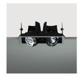
rectangular recessed luminaire with 2 optical assemblies - warm white passive dissipation LEDs - integrated electronic control gear - flood
