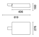
Pole-mounted system - Large body optical assembly - Warm White - A45 street optic.
