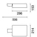
Pole-mounted system - Small body optical assembly - Warm White - ST1 street optic.
