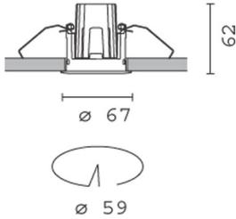
**Adjustable (tilting) round recessed luminaire - LED - spot**
