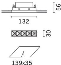
**5 cell Frameless Recessed luminaire - Tunable White - Flood optic**
