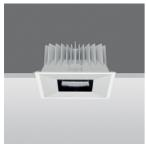
Square recessed luminaire - 226x226 mm H=103 mm - neutral white - DALI ballast - general light optic with controlled luminance UGR<19
