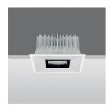
41 212x212 Square recessed luminaire - 226x226 mm H=103 mm - LED neutral white - DALI ballast - general light optic with controlled luminance UGR<19
