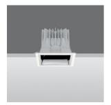
Square recessed luminaire - 144x144 mm H=111 mm - LED neutral white - electronic ballast - general light optic with controlled luminance UGR<19
