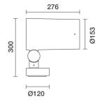
Spotlight with base - Neutral White Led - integrated electronic control gear - Very Wide Flood optic Photometric data for this product will be available starting from September 2018.
