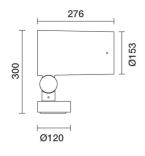
Spotlight with base - Neutral White Led - integrated electronic control gear - Wide Flood optic Photometric data for this product will be available starting from September 2018.
