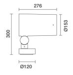
Spotlight with base - Warm White Led - integrated electronic control gear - Wide Flood optic etric data for this product will be available starting from Septe
