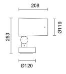
Spotlight with base - Neutral White Led - integrated electronic control gear - Very Wide Flood optic Photometric data for this product will be available starting from June 2018.
