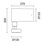
Spotlight with base - Warm White Led - integrated electronic control gear - Very Wide Flood optic Photometric data for this product will be available starting from September 2018.
