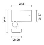
Spotlight with base - Neutral White Led - integrated electronic control gear - Flood optic etric data for this product will be available starting from September 2018
