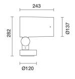
Spotlight with base - Warm White Led - integrated electronic control gear - Super Spot optic etric data for this product will be available starting from Septe
