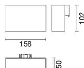
**Wall-mounted Laser Blade InOut, Warm White LED, Wide Flood optic****Product code**
