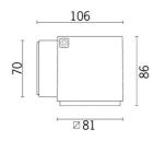
Outdoor wall-mounted luminaire - Warm white LED - with electronic ballast Vin=100-240V ac - Flood optic
