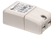
Code: 150 Supported n. of lamps: 1 Power supply dual function Vout 24Vdc: 8W/100÷240V Iout 350mA: 6X1W/100÷240V IP20 CLASS II SELV EQ.
