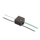
Code: 237 SPD: (Surge Protection Device) 275Vac Maximum discharge current 10KA (8/20µs) Maximum operating current 5A Suitable for series connection - IP66
