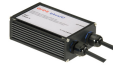
Code: 141 Supported n. of lamps: 10 Power supply with DMX interface for RGB fixtures 36W/220÷240V-3CHx350mA (3CHx10x1W) DMX control allowed IP67 CLASS I SELV EQ.
