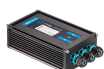
Code: 218 Supported n. of lamps: 12 Power supply 13X2W/110÷240V - Iout 500mA (7X2W@110V) IP67 CLASS II SELV.
