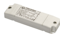
Code: 68 Supported n. of lamps: 10 Power supply 10x1W/100÷265V - Iout 350mA (7x1W@110V) IP40 CLASS II SELV EQ.
