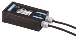
Code: 147 Supported n. of lamps: 5 Power supply 20W/220÷240V - 24Vdc IP67 CLASS II SELV.
