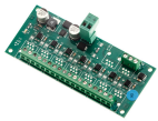
Code: 187 DMX splitter Electronic device to regenerate the DMX signal. 1 input and 7 output. 12÷24Vdc Power supply to be ordered (87 or 175 recommended)
