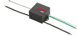
Code: 237 SPD: (Surge Protection Device) 275Vac Maximum discharge current 10KA (8/20µs) Maximum operating current 5A Suitable for series connection - IP66
