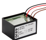
Code: 106 Supported n. of lamps: 1 Power supply dual function Vout 24Vdc: 8W/100÷240V Iout 350mA: 6X1W/100÷240V - IP65 CLASS II SELV EQ.
