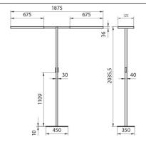
LED light source work equipment electronic ballast connected load 220-240V, 50/60Hz power consumption env. 200 W power factor env. 0,966 luminous flux approx. 28.500 lm
