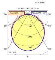
Light sourceLEDWork equipmentWithoutConnected load22 - 26 V; DCPower consumptionca. 21 WLuminous fluxapprox. 520 lm
