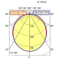
Light sourceLEDWork equipmentWithoutConnected load22 - 26 V; DCPower consumptionca. 13 WLuminous fluxapprox. 325 ImLuminous efficiencyapprox. 25 Im/W
