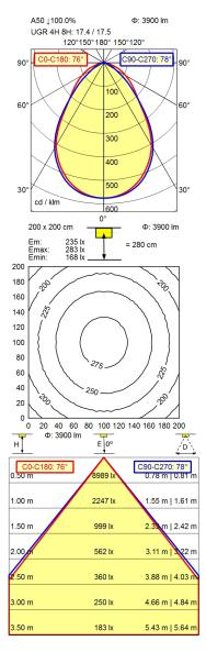
Work equipment Electronic ballast **Connected load** 220 - 240 V; 50 Hz; 60 Hz Power consumption ca. 30 W Standby ca. 0,5 W Power factor env. 0,900 Luminous flux approx. 3.900 lm Luminous efficiency approx. 130 lm/W Light type/-color Warm white Colour temperatur approx. 3.000 K Color rendering index CRI ≥ 80 Light distribution Direct **Direct ratio** approx. 100 % Beam angle 76° / 78° **Chromaticity tolerance LED** < 3 SDCM
