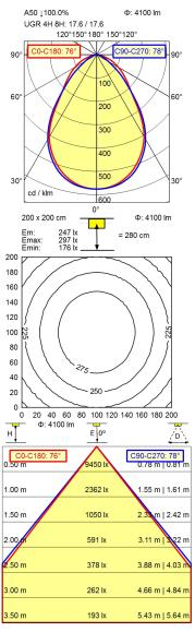
Work equipment Electronic ballast Connected load 220 - 240 V; 50 Hz; 60 Hz Power consumption ca. 30 W Standby ca. 0,5 W Power factor env. 0,900 Luminous flux approx. 4.100 lm **Luminous efficiency** approx. 136 lm/W Light type/-color Cold white Colour temperatur approx. 4.000 K Color rendering index CRI ≥ 80 **Light distribution** Direct **Direct ratio** approx. 100 % Beam angle 76° / 78° **Chromaticity tolerance LED** < 3 SDCM
