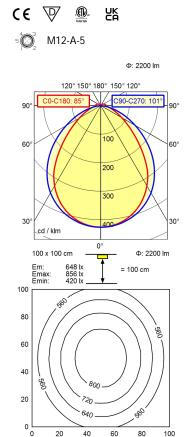
Light source LED Work equipment Without **Connected load** 22 - 26 V; DC **Power consumption** ca. 17 W Luminous flux approx. 2.200 lm Luminous efficiency approx. 129 lm/W Light type/-color Cold white Colour temperatur approx. 5.000 K Color rendering index CRI ≥ 80 Light distribution Direct Beam angle 85° / 101° **Chromaticity tolerance LED** < 4 SDCM Glare control Screen System of protection IP 54
