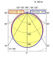
Light sourceLEDWork equipmentWithoutConnected load22 - 26 V; DCPower consumptionca. 12 WLuminous fluxapprox. 260 lmLuminous efficiencyapprox. 21 lm/W
