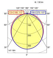
Light sourceLEDWork equipmentWithoutConnected load22 - 26 V; DCPower consumptionca. 6 W
