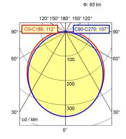
Light sourceLEDWork equipmentWithoutConnected load22 - 26 V; DCPower consumptionca. 3 WLuminous fluxapprox. 65 ImLuminous efficiencyapprox. 21 Im/W
